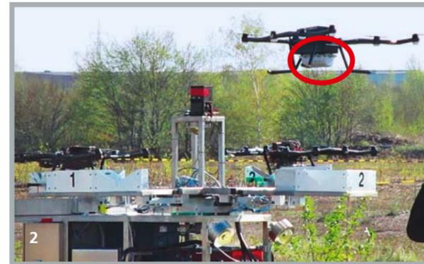
a picture of the situation. This UAV stayed in position while a second, fitted with a radioactivity sensor, was flown in. The second UAV followed a predetermined path that allowed the fastest and most effective search of the area, thus fixing the precise position of the source.
